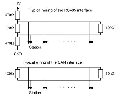
The resistances shown are built into the detector and can be enabled using DIP switches.  $\rightarrow$  3.5.2, RS485 interface bus termination  $\rightarrow$  3.5.3, CAN bus termination
