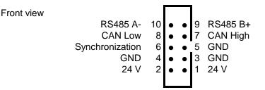
The ribbon cable connection is used to synchronize the detectors with each other and to provide the supply voltage and interface connection. The supply and interface connection to the control device can be made either using the ribbon cable or a plug terminal (see 6.1, Plug terminal: Supply and interface).
