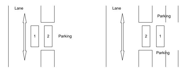
The placing of the loops depends on which travel direction backups are anticipated in. In travel direction  $1 \rightarrow 2$  no backups are permitted! In travel direction  $2 \rightarrow 1$  even vehicles in traffic line situations are correctly counted, whereby the vehicle gap must always enable a loop.
