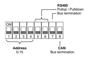
Note! Before startup check all DIP switches for the correct position! Improper setting can damage the interfaces.
