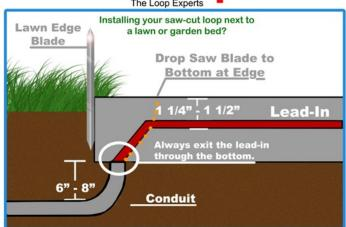
Lead-in should be run 6"-8" below the surface. Always run the lead-in through conduit
